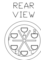
INLINE: 6-PIN INLINE SOCKET INSERT (FEMALE)
