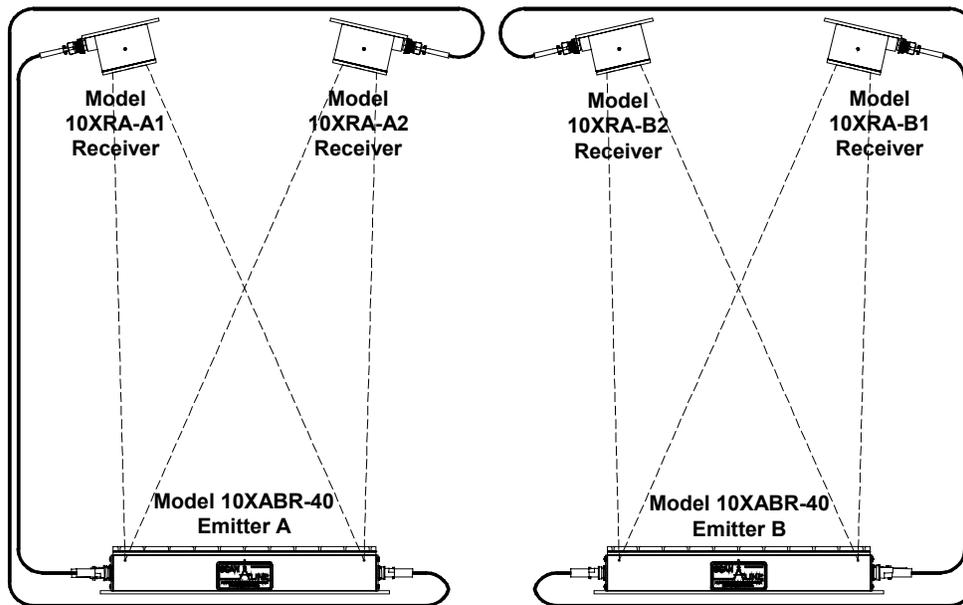
Figure G.1-1: Model 10XABR-40 Dual-Sensor System for Passline Independent Width Measurement
