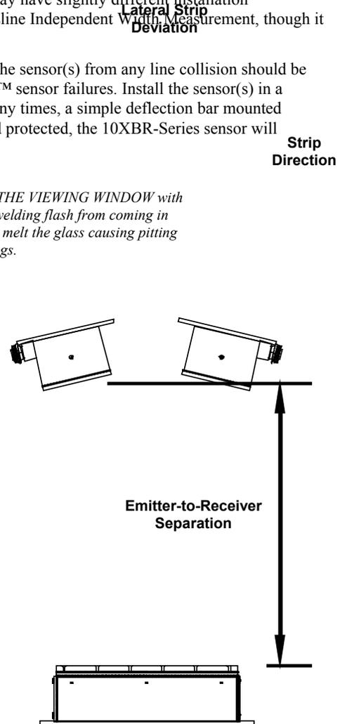
Figure G.4-1: Emitter-to-Receiver Separation
