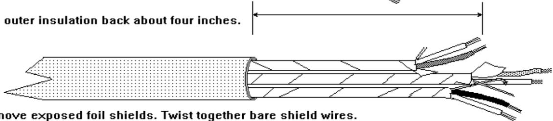
3. Remove exposed foil shields. Twist together bare shield wires. Cut off shield wires at one inch length.
