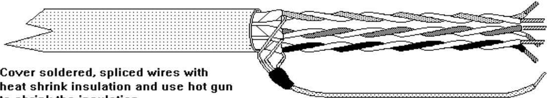
5. Cover soldered, spliced wires with heat shrink insulation and use hot gun to shrink the insulation.
