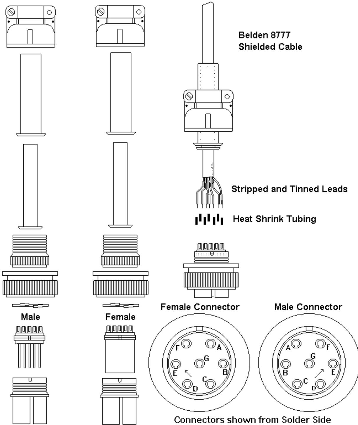
Figure G.6-2: Exploded View of Standard Enclosure 7-Pin Cable
