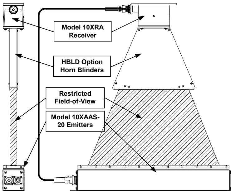
Figure G.5-3: Field of View with Model 10XAAS-20 Sensor and Horn Blinder
