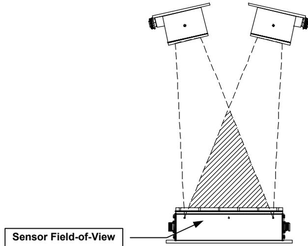
Figure G.4-6: Sensor Field of View
