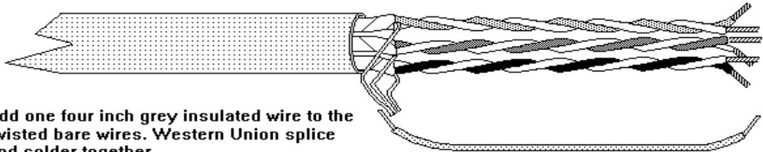
4. Add one four inch grey insulated wire to the twisted bare wires. Western Union splice and solder together.
