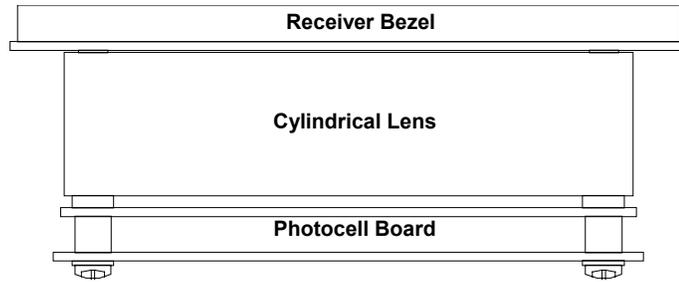
Figure G.1-4: Model 10XRA Receiver Interior View
