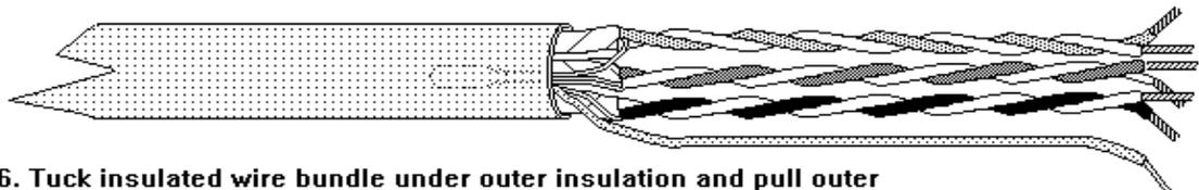
6. Tuck insulated wire bundle under outer insulation and pull outer insulation back over the exposed inner wires.
