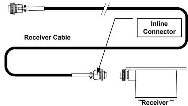
Figure G.6-3: 10X Receiver with Cabling
