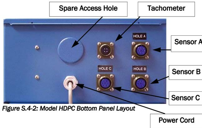
Figure S.4-2: Model HDPC Bottom Panel Layout
