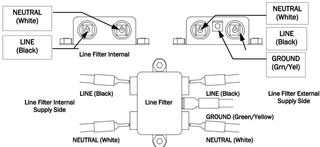
Figure S.4-1: Line Filter for AC Power Connection in Model HDPC
