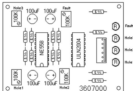
Figure S.4-4: Quad Relay Extender Option Board
