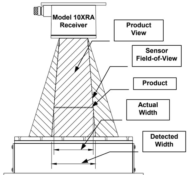
Figure ZC.8-1: Sensor and Product Views with Model 10XAAS-10 Sensor
