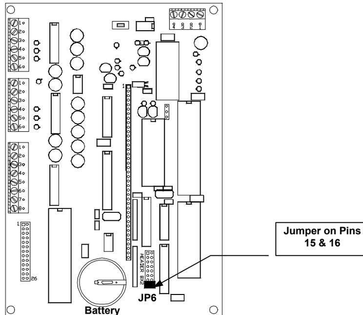
The jumper for the Model MPPU Level 3 customer interface should be located on pins 15 and 16 {Figure ZC.1-3} of the Model MPPU micro-controller board (Part # 3695172 Rev. C).
