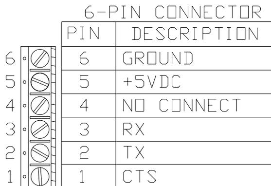
Figure ZC.15-1: LED Keypad/Display Connections
