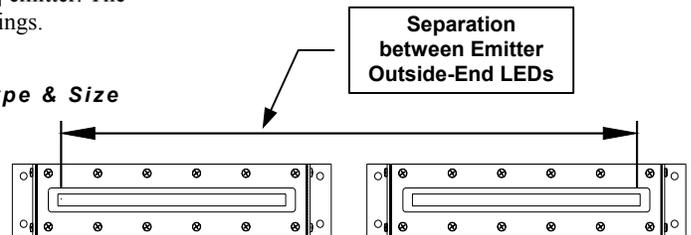
Figure ZC.7-1: Outside-End Emitter LED Separation
