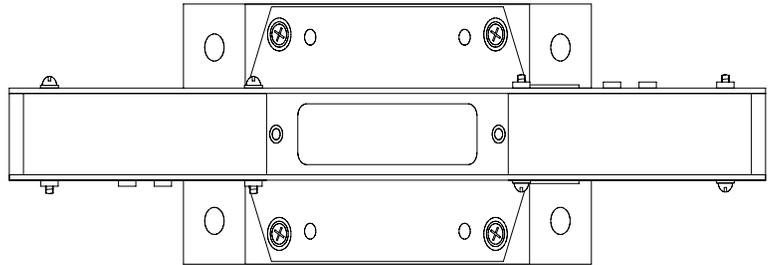
**Figure E.5-7: Horn Blinder Properly Aligned on Model SHD-4000-Series Receiver**
