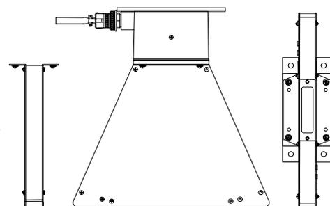
Figure E.5-1: HBLD Option Installed on Model SHD-4000R-Series Standard Duty Receiver
