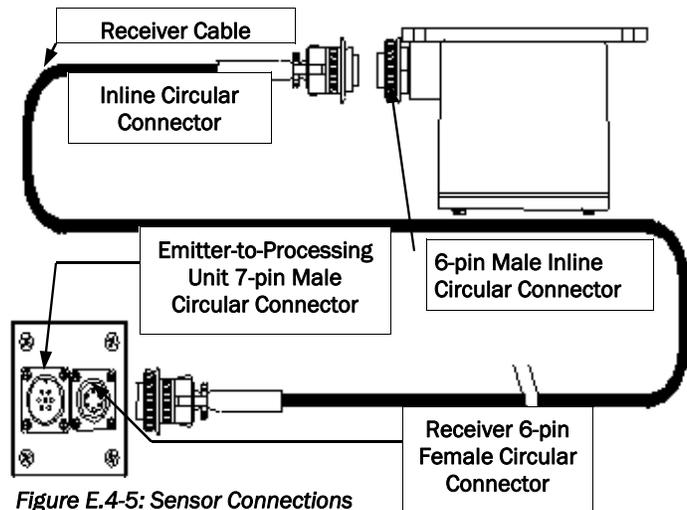
Figure E.4-5: Sensor Connections
