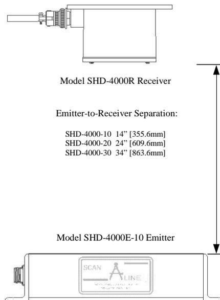
Figure E.4-2: Sensor Separation for SHD-4000-Series Sensors
