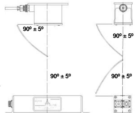
Figure E.4-1: Emitter-to-Receiver Alignment
