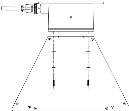
**Figure E.5-6: Horn Blinder Screw Assembly on Model SHD-4000-Series Receiver**
