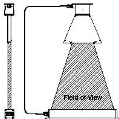
Figure E.5-2: Field of View with Model SHD-4000-20E-B Standard Duty Sensor with Horn Blinder
