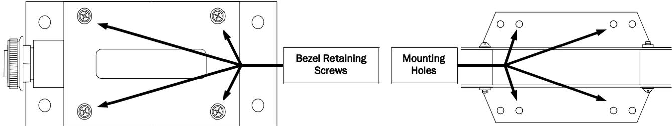
**Figure E.5-4: Model SHD-4000R Bezel Retaining Screws**
